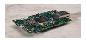
16 or 64 core Epiphany co-processor Gigabit Ethernet 2x USB ports + HDMI port
