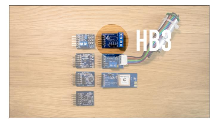
GPIO H-bridge Driver with Feedback Inputs Drive a DC motor with operation voltage up to 12V
