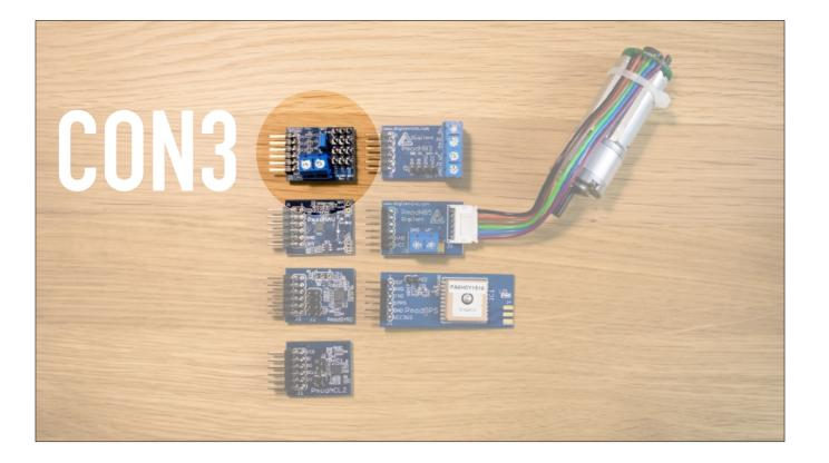
GPIO Four standard 3-wire servo motor connectors
