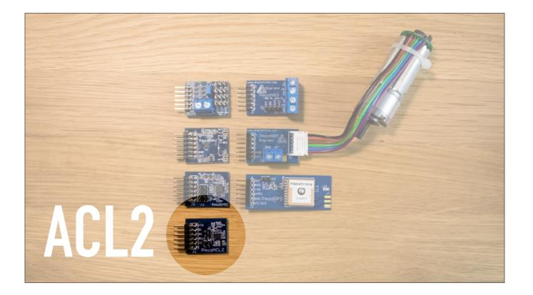
SPI 3-axis Microelectromechanical System (MEMS) Accelerometer
