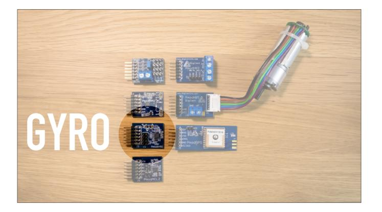
SPI 3-axis Digital Gyroscope
