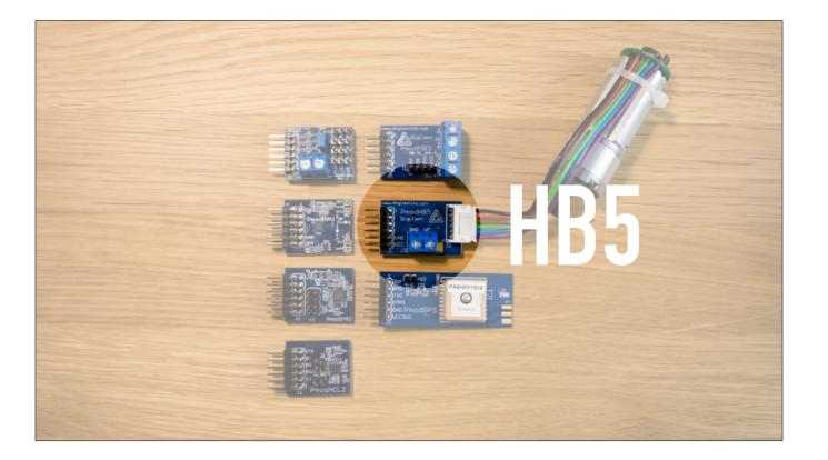
GPIOH-bridge Driver with Feedback Inputs6-pin JST connector for direct connection to Digilent motor/gearboxesDrive a DC motor with operation voltage up to 12V
