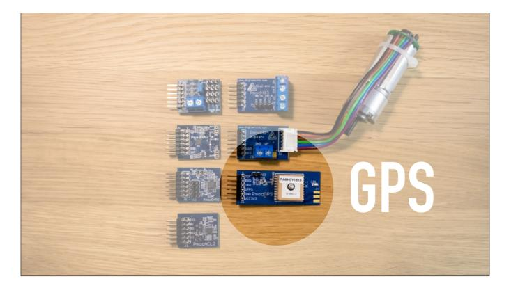
UART GPS Receiver 3m 2D satellite positioning accuracy
