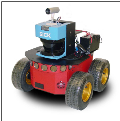
Figure: A Pioneer 3-DX with a laser sensor and a video camera
