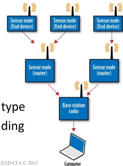
You change device type by loading corresponding firmware
