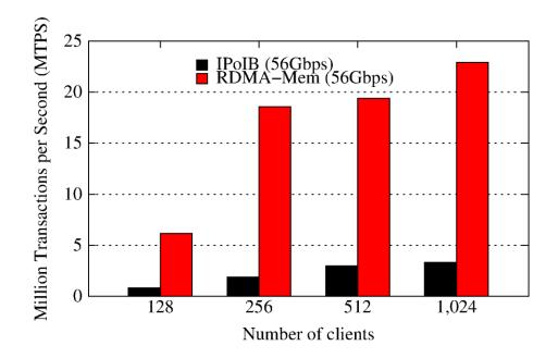
Memcached performance comparisons of TCP v. RDMA 36 node cluster, 32 requesters, 4 servers Same physical 56Gb network interface used in both cases Running RDMA enhanced memcached, in-memory mode, 4KB message size
