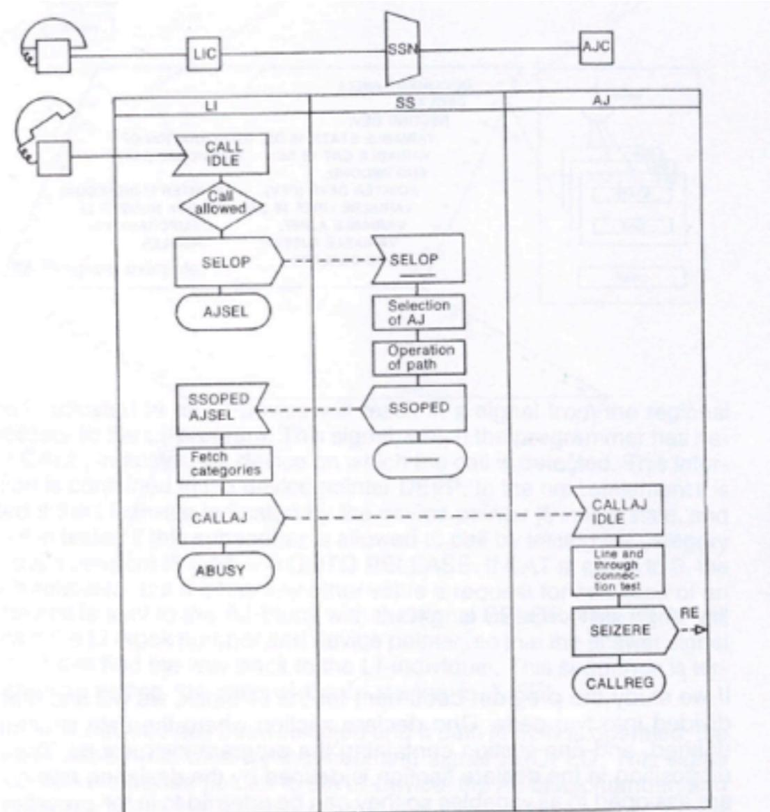
Fig. 11 AXE programming by PLEX
